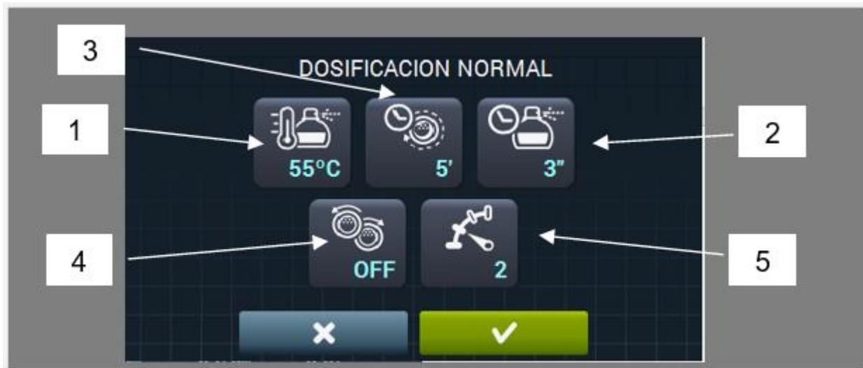
1. **Objective dispenser temperature (°C/°F)** As soon as the temperature falls below this temperature, the dispensing operation will take place.
